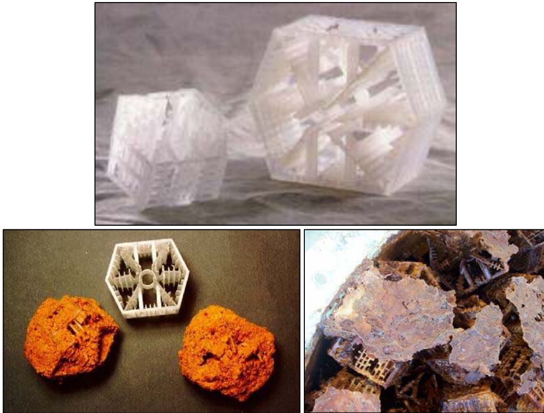
Figure 2 – Examples of packed tower media both clean and fouled.
