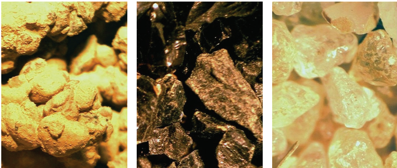
Figure 1 - Microscopic images of fouled filter media before (left) and after (center, right) Floran® treatment
